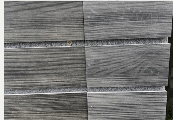
Left: Sealed Sample Kept Indoors for 8 Months Right: Sample After 8 Months Outdoor Exposure
